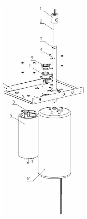
Figure 8. Hot and cold tank assembly.
