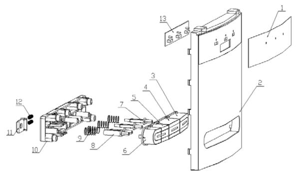
Figure 9. Faucet and front hatch assembly.
